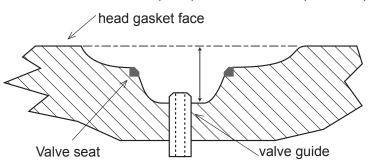
standard volume check can be carried out, in which case you would expect to read a minimum of 21.2cc. If this value is not obtained then a full inspection would be needed using the gauges and measuring methods to decide the eligibility of the engine. The head gasket face may be machined, but the cylinder head must at all times comply with all of the gauges and dimensions.
