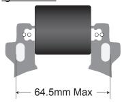
The ignition coil (including ignition lead) will be the standard and unmodified unit. Either original or later type coil can be used. The coil mounting bolts must be standard and unmodified and use the original mounting positions (see also section 23 concerning welded repair).
