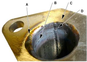
The rippled weld (A) should be clearly visible around the complete inside of the flange, and only be violated or interrupted where linishing has taken place across the flange plate (C). Outer weld penetration (B) should also be visible. The inner seam of the exhaust tube (D) should be visible, original and undamaged.
