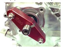
the split should have its edge resting on the magnet mounting. If it rests on the magnet, it is non-compliant.
