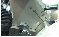
rotated against the location tool in a clockwise direction (flywheel side) before the reading is observed on the template tool. The standard and unmodified fan must be used, with all fins in place.
