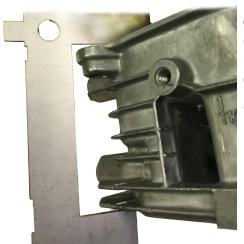
When placing the CPO gauge over the rocker cover face, the lower lip must not engage over the cylinder mating face
