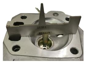
The spark plug insert must show a clearance to the CPO gauge, which must be flush on the cylinder face
